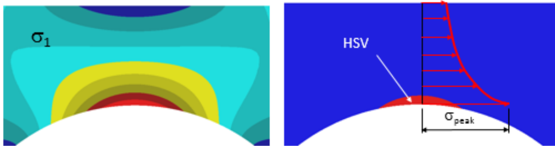
Figure 6: Example of the stress distribution around a circular cutout in a test specimen (left) and the corresponding size of the HSV computed using Eq. (28) with \gamma = 0.85 (right).
