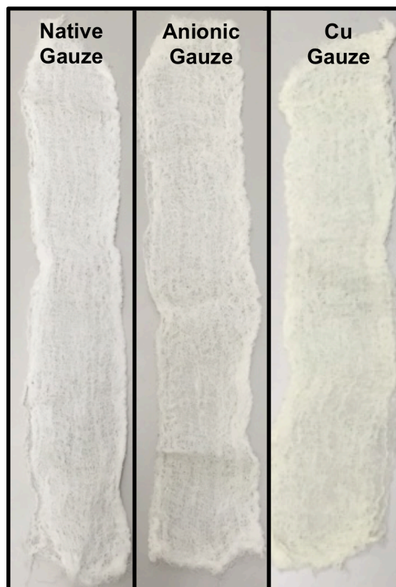
Figure 3. Photographs of the prototype cotton gauze dressing taken throughout the coating process.
