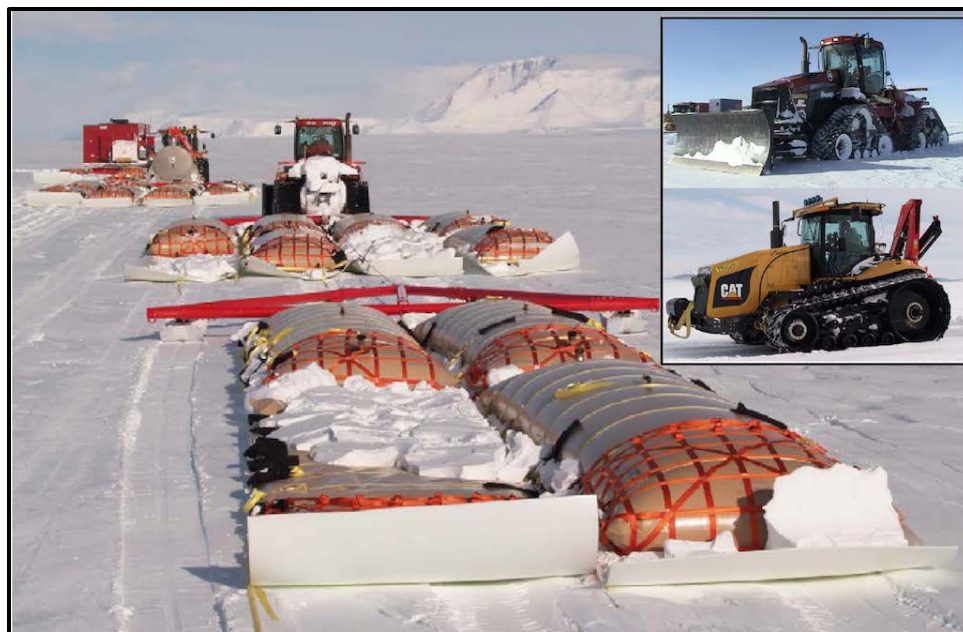
Figure 1. Portions of the SPoT caravan shown hauling modified fuel-bladder sleds along the traverse route. Inset shows two rubber-tracked, agricultural tractors used on SPoT (Case Corporation and Caterpillar). (Adapted from Lever and Thur 2014.)
