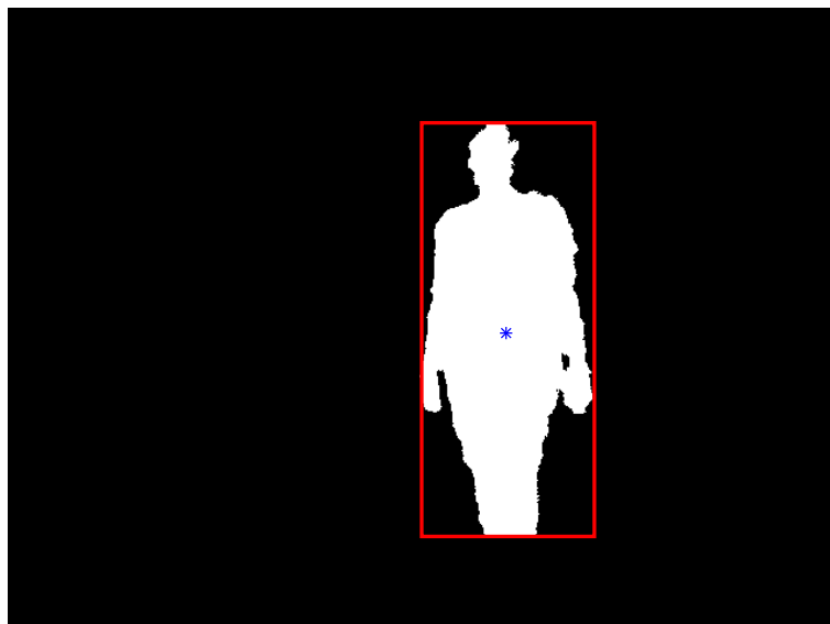
Figure 33. Image Segmentation Result with Two Individuals at Different Depths
