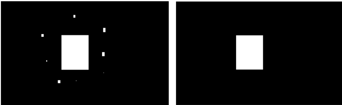
Figure 17. Opening of an Image with 20x20 Square Structuring Element to Eliminate Clutter
