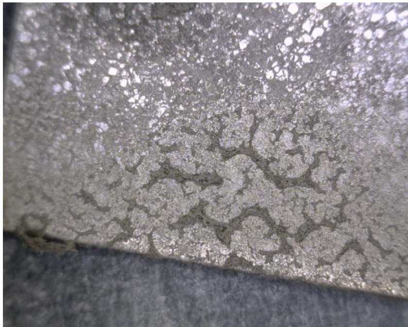
Optical microscopy of sample 35 reveals areas that have been coated with the reduced nickel particles and areas that have not been coated.
