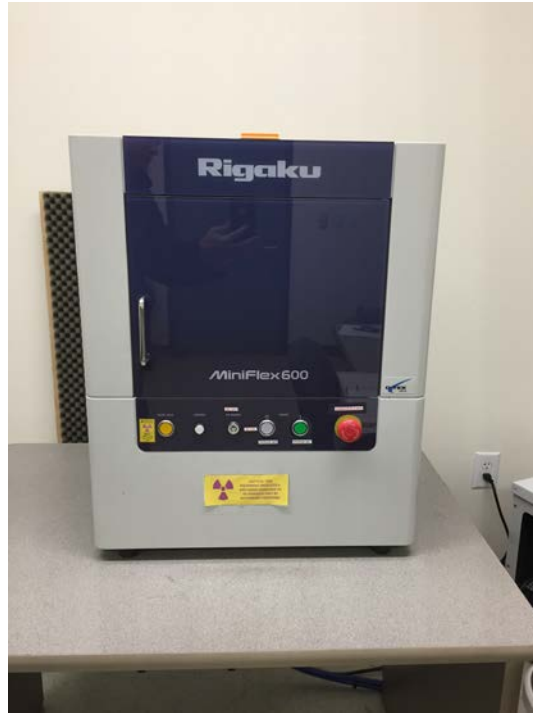
The Rigaku MiniFlex 600 was used to characterize the powders to identify the material composition.
