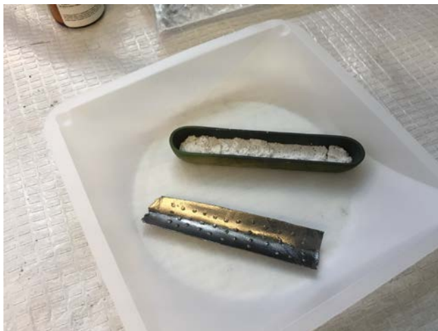
Lignite and potassium carbonate mixture were placed in the crucible with a perforated piece of graphite foil.
