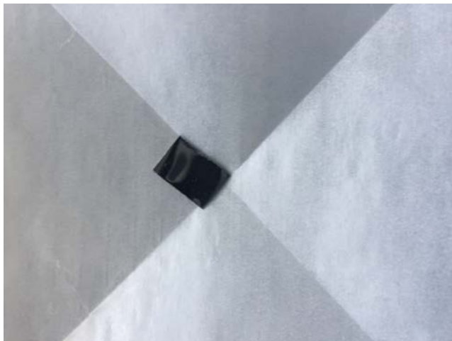
Iron foil sample after being polished with POL metal polish.
