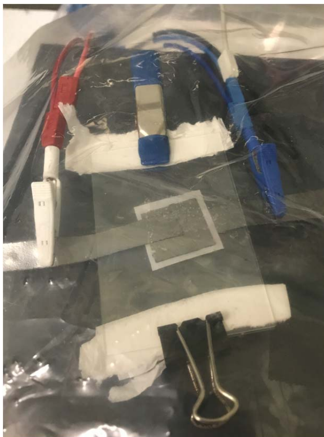
Figure 14. PSDM Capacitor Connected to the VSP 300 Leads Ready for Testing
