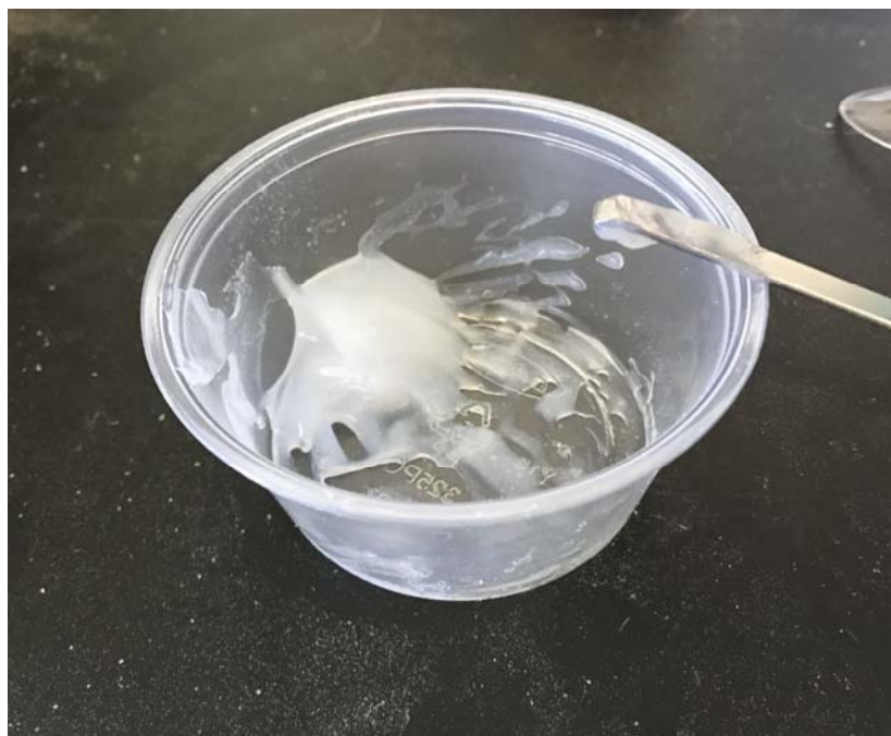
Figure 10. Fumed Silica PSDM Mixture after Mixing
