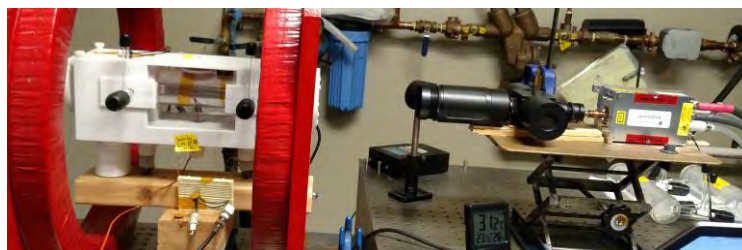
Fig. 1. SEOP setup using a 125 W narrowed laser (QPC), collimating-polarizing optics (black), 3D-printed forced-air oven 7 (white) with interior NMR detection coil, 2" diam. OP cell in red Helmholtz pair magnet, and low-frequency NMR spectrometer (Magritek Aurora, not shown).
