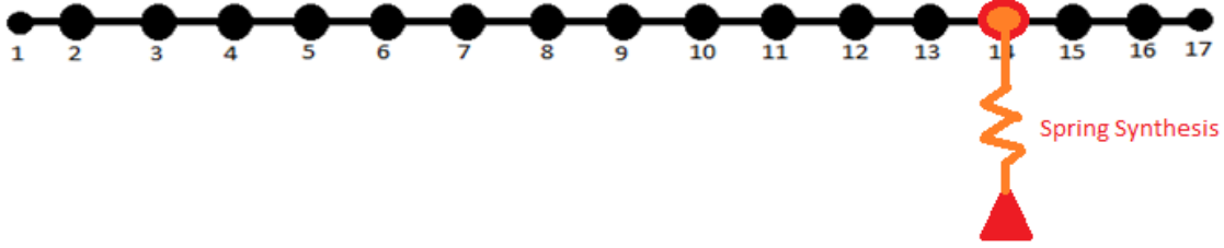
Figure 7. 16-Element Structure with Artificial Spring.
