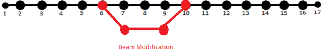
Figure 5. 16-Element Structure with Beam Modification.
