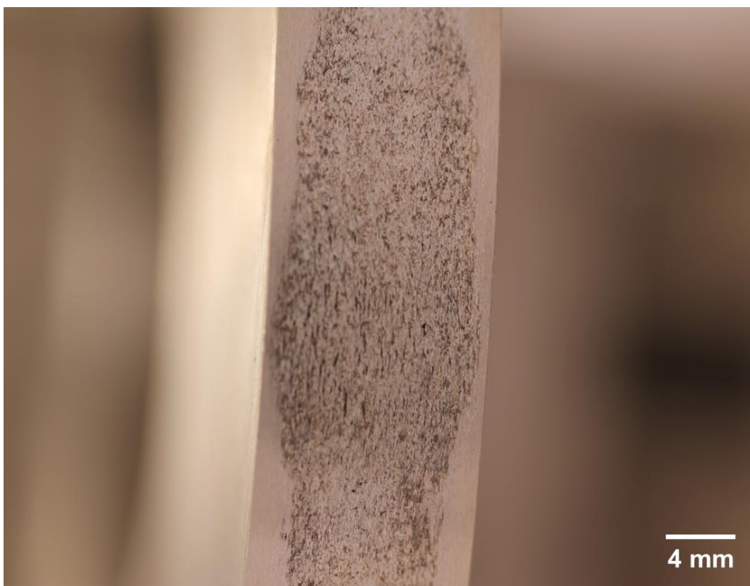
Figure 61 – RCF test results showing scuffing surface on the carburized 8620 steel roller.
