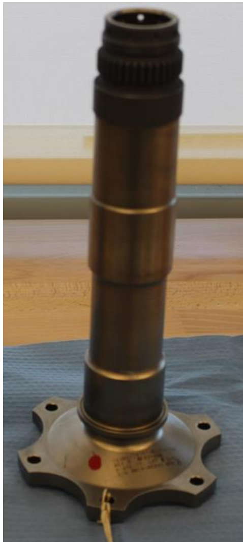
Figure 33 – Cooling fan shaft for AH64 identified by CCAD as a Critical Parts Demand item DDM repair candidate.
