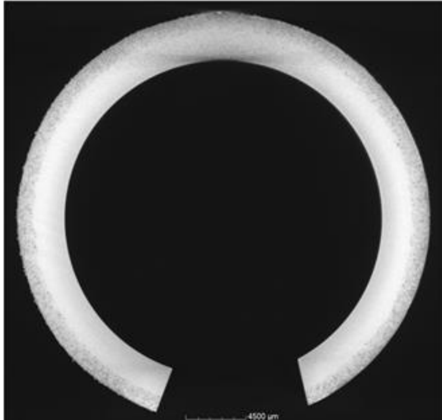
Figure 41 – Radiographic-based tomography of cooler fan shaft.
