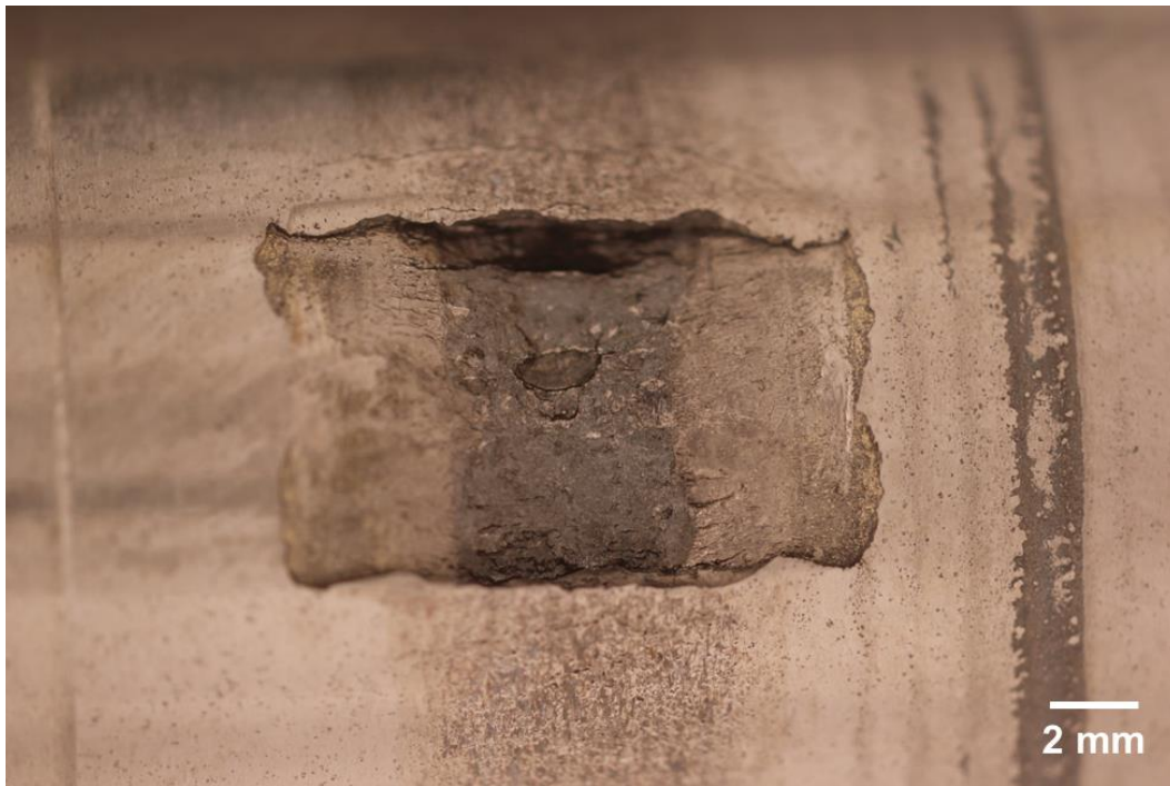
Figure 62 – RCF test results showing surface pitting on the SS 431/20 TiC specimen.
