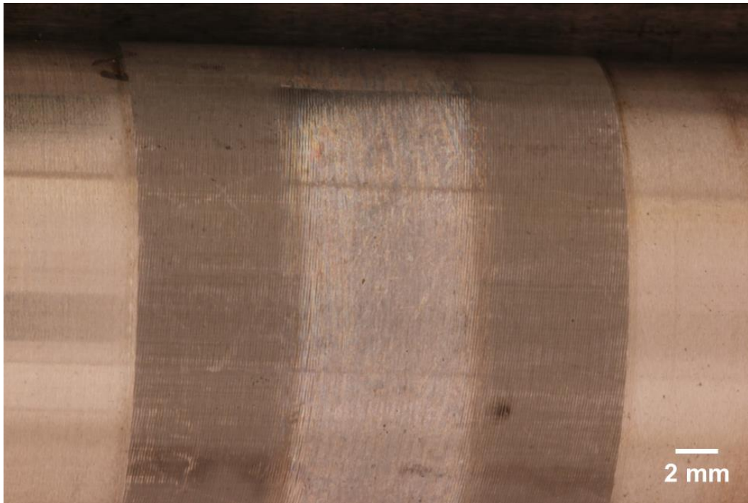
Figure 64 – RCF results of the carburized 8620 steel specimen without scuffing surface.
