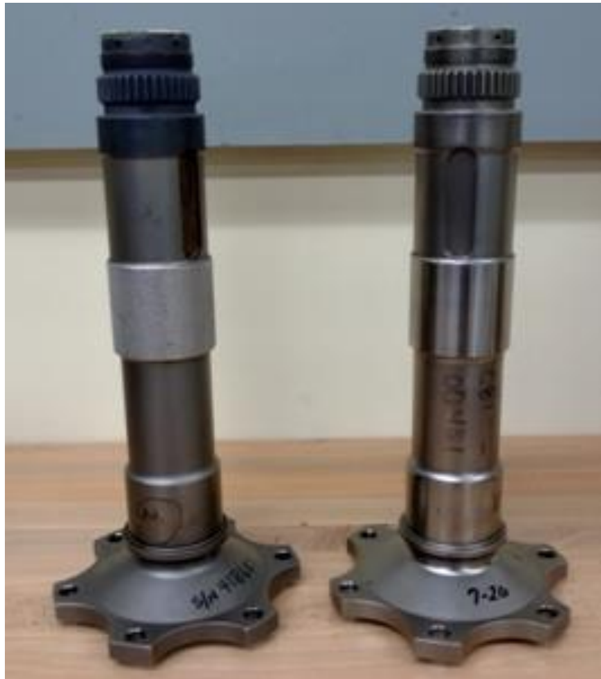
Figure 44 - Post-process machining and dimensional inspection cooler fan shaft.
