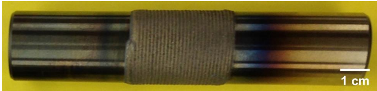
Figure 28 – Carburized 8620 steel specimen that had been laser deposited with SS 431/20 TiC.
