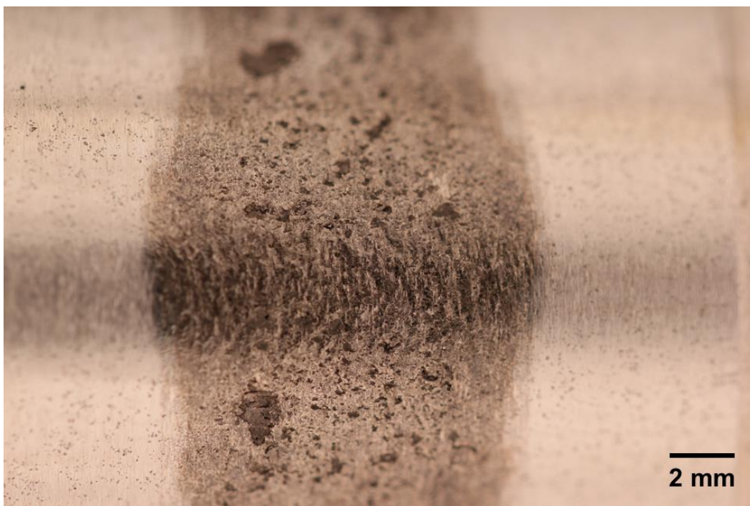
Figure 60 – RCF test results showing scuffing surface on the SS 431/20 TiC.
