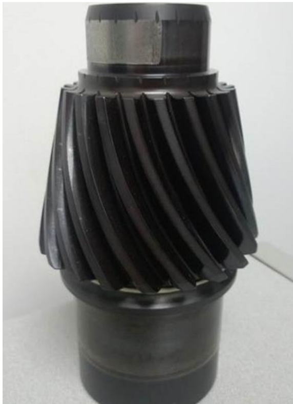
Figure 32 – Input pinion for AH64 identified by CCAD as a Critical Parts Demand item DDM repair.
