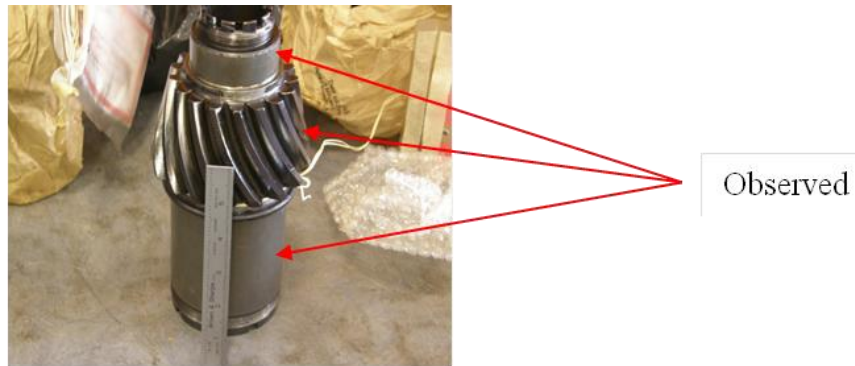
Figure 46 – H60 pinion gear faults.
