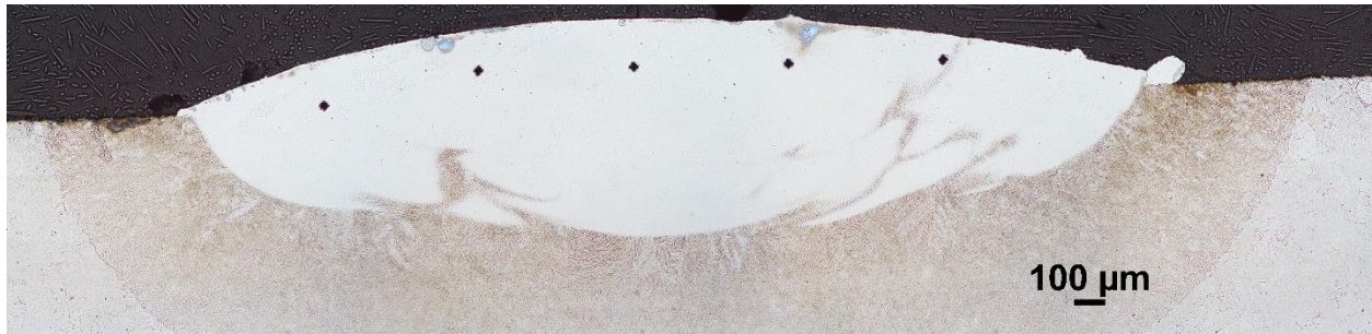
Figure 25 – Single track deposit of SS 431 at 1.0 cm 3 /min powder flow rate and 2 kW laser power.
