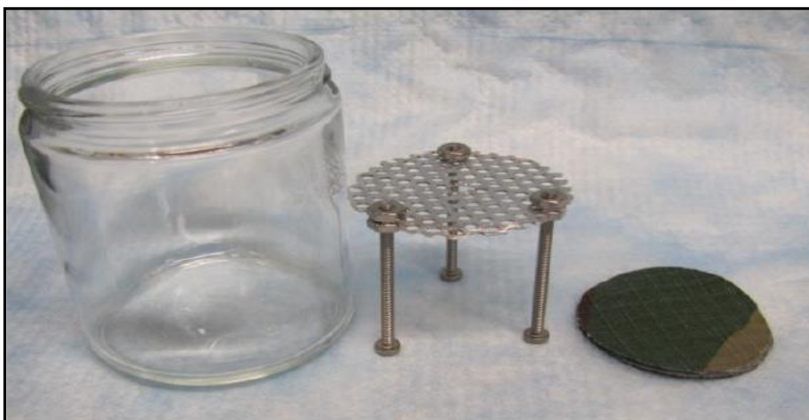
Figure 3. Swatch preconditioning jar, mesh platform, and sample swatch.
