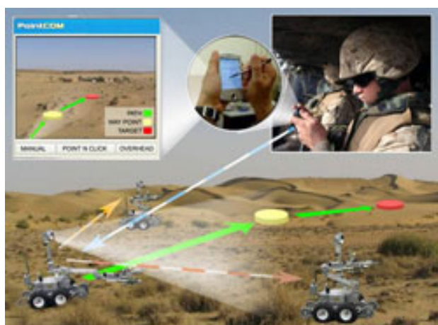
Figure 9-3: Vehicle Intelligence Involves Multiple On-Board Sensors, Autonomy Algorithms, and Interaction with Remote Operators and Resources.
