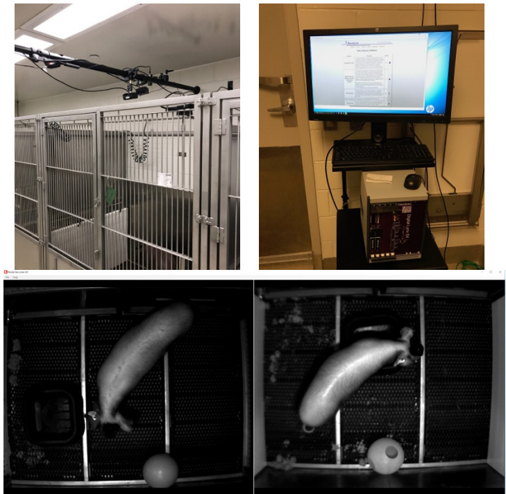
Fig. 6. Pig Epilepsy Monitoring Unit (EMU). Images above demonstrate the video acquisition using IR for 24 hour recordings/monitoring of the pigs (2 shown). Also depicted is the acquisition system for the wireless data, as well as the home cage with the IR illuminators, cameras, and wireless hubs.
