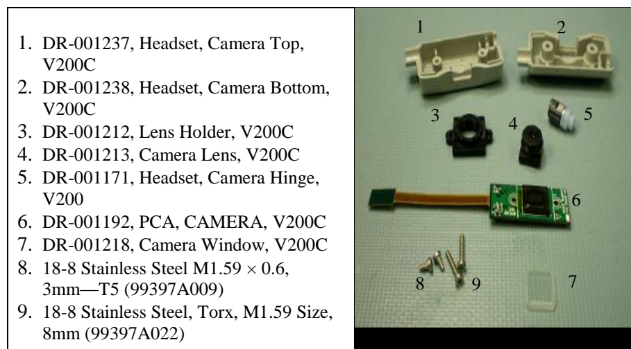
Figure 1. BrainPort V200 Camera Assembly
