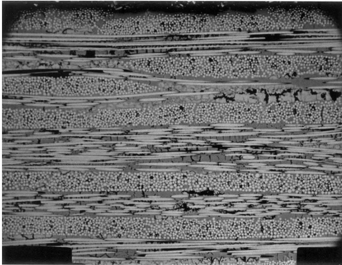
Figure A-1.1.3: Micrograph of 2-D S200, 80 mil @ 50x, AB. This figure illustrates the excellent infiltration of fiber tows in the 2-D material.
