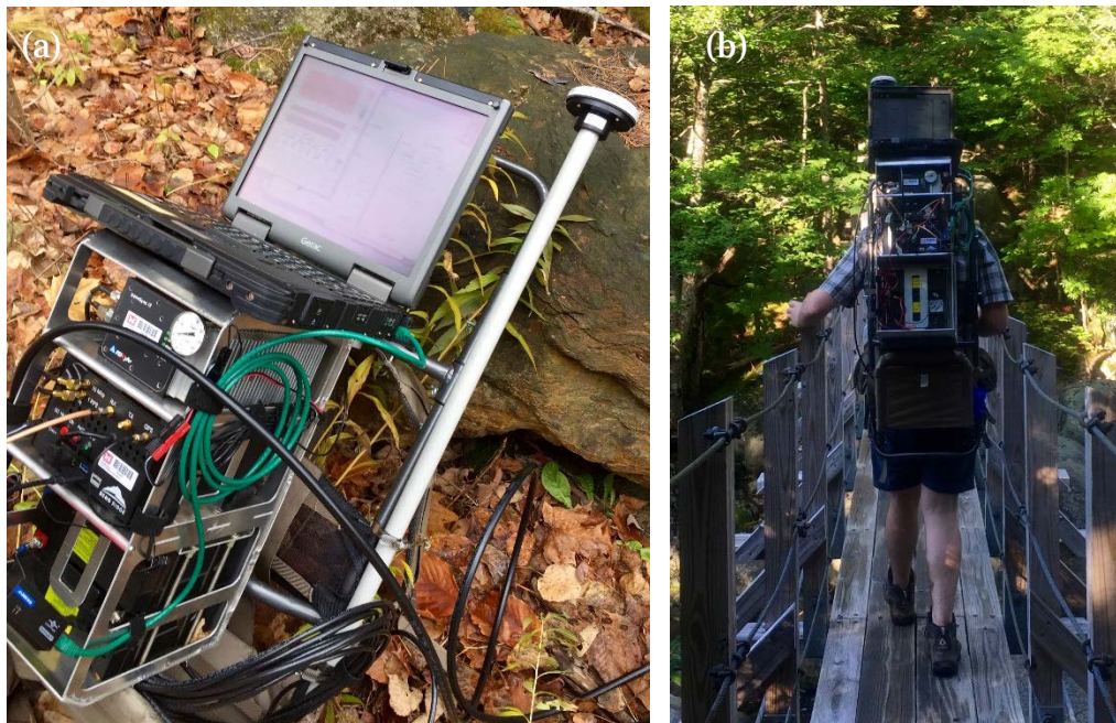
Figure 1. The 23 kg station backpack: (a) from top to bottom, Getac B300 field laptop; external Rb clock; mWISP unit; two solid-state, 24 VDC, 10 A-h LiFePO 4 batteries; and GPS antenna on the right and (b) the station backpack shouldered for transport.
