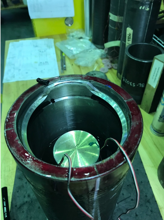
Figure 5: Wedge Ring Failure Shown in Tube
