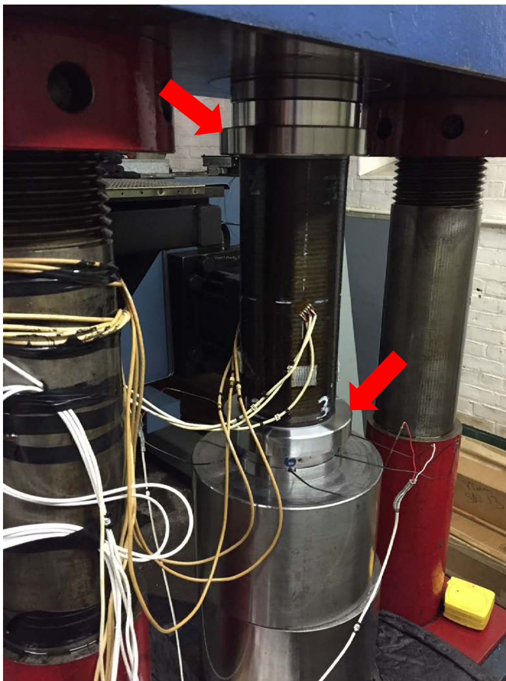
Figure 7: PMC Test Setup with Dilation Limiting Rings
