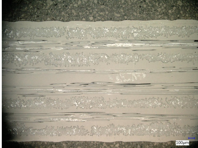
Figure 2. Optical micrograph of HiPerComp™ Gen 1.1 Hi-Nicalon/SiC (0/90)2s showing a 0/90 cross-section at 100×
