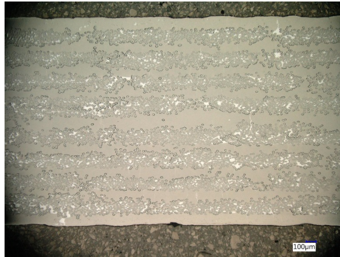
Figure 6. Optical micrograph of HiPerComp™ Gen 1.1 Hi-Nicalon/SiC (0/90)2s showing a \pm 45 cross-section at 100×
