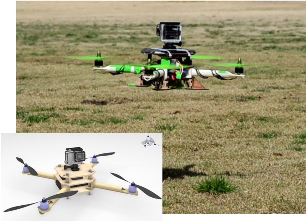
Figure 39: Tailored Design for Bridge Inspection
