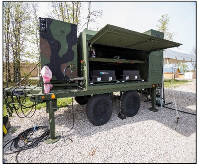
Figure 41: Hybrid Power Trailer
