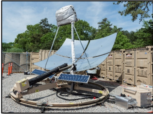
Figure 7: SPSWH Including Water Pump and Battery Pack
