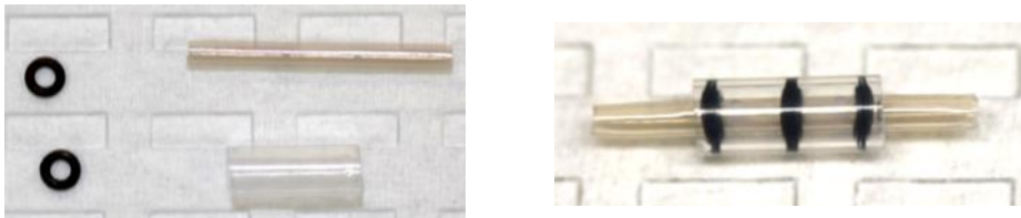
Figure 2. (left) Conduit Components - inner conduit, outer conduit, and end caps (right top) Inner conduit with two end caps defining the outer boundary of the reservoir (right) Completed PTFE device with inner and outer tube, as well as a diffusion hole on the inner conduit that enables the release of drug from the reservoir into the inner chamber (bottom)
