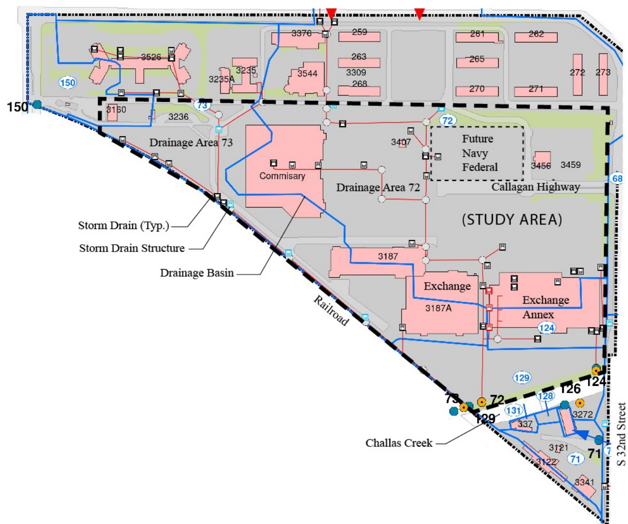
Figure 1-3: Project Drainage Areas and Storm Drain Infrastructure
