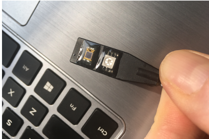
Figure 3 – Upgraded OXT5 sensor covered by an additional layer of clear silicon.
