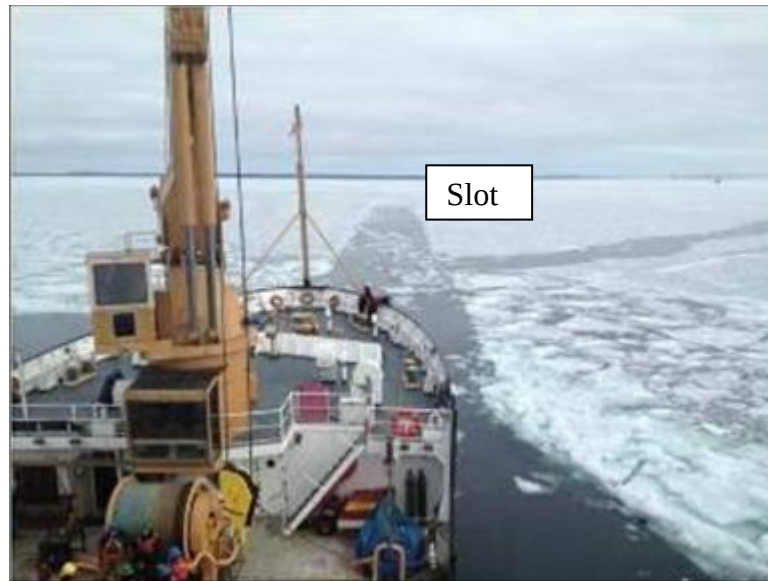
Figure 11. Channel or ‘slot’ created in sheet ice to facilitate oil skimmer deployment.
