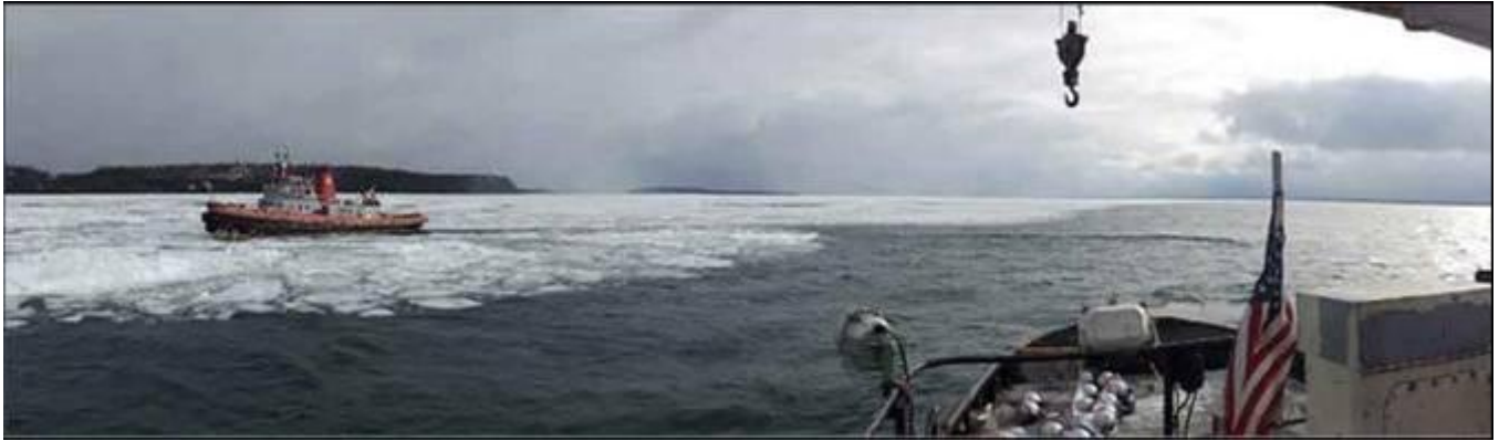
Figure 18. Fire Boom (PyroBoom™) deployed and towed by two tugboats to simulate collection of oil in rubble ice.
