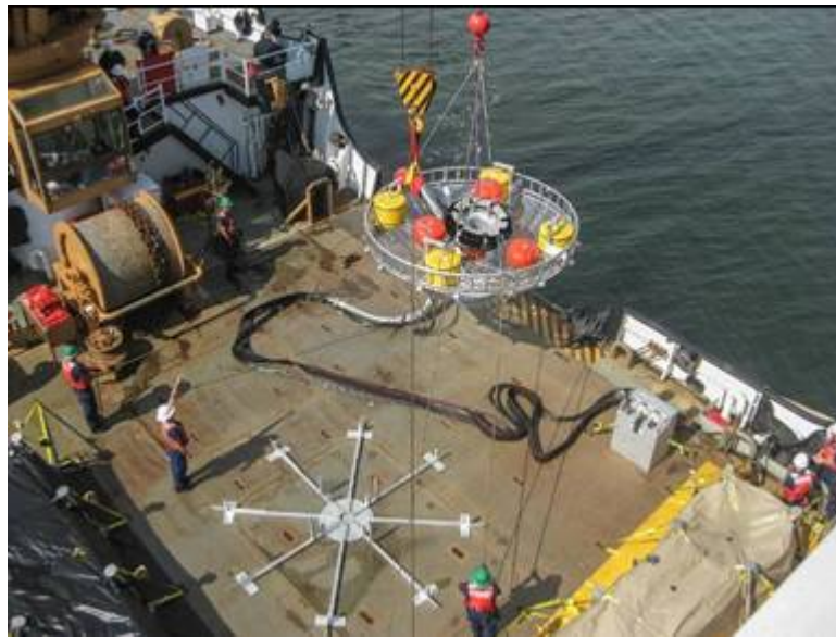
Figure 23. Ice cage integrated with a DOP-Dual Helix skimmer.
