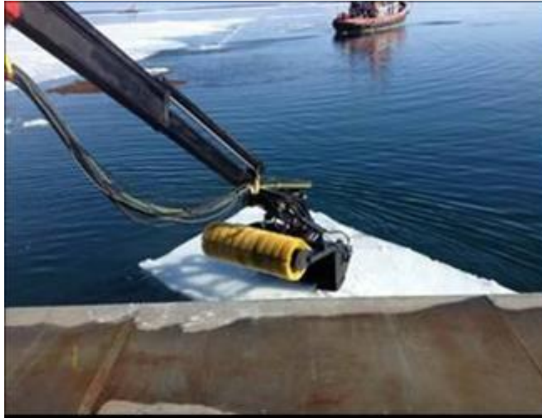
Figure 17. LRB demonstrating ability to push ice out of way.
