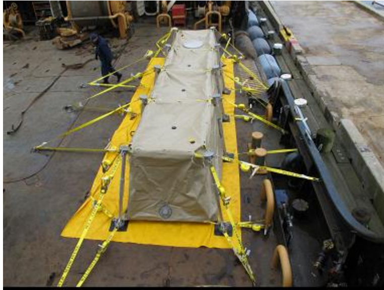
Figure 20. Empty, collapsible TST ready for service.
