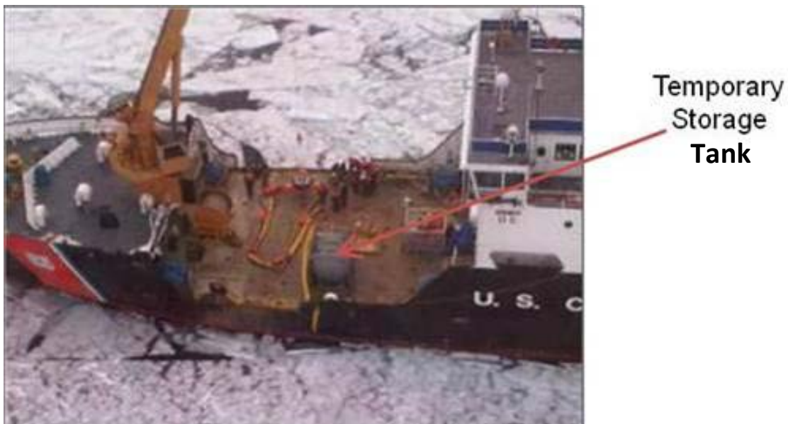
Figure 19. A temporary storage tank mid-deck on a Juniper Class Seagoing WLB.
