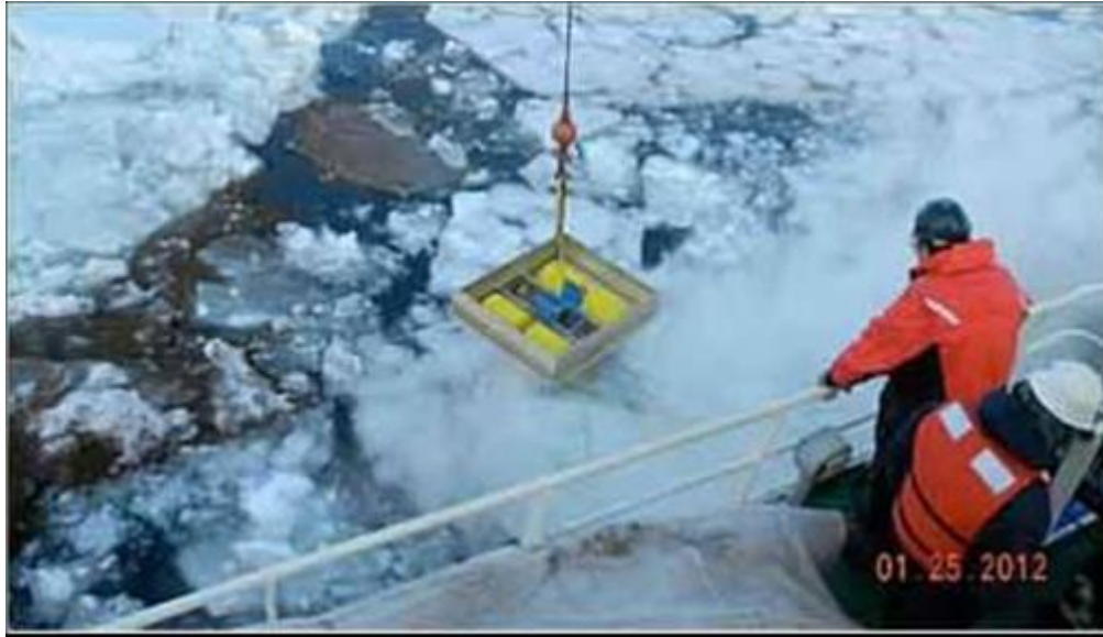
Figure 14. Drum skimmer deployed in rubble ice.
