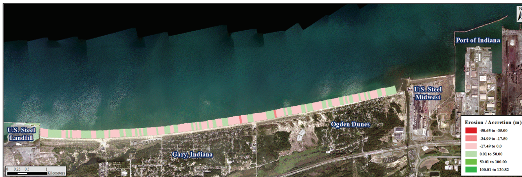
Figure 8. Shoreline change from the Port of Indiana to the U.S. Steel Landfill from 2012 to 2014.
