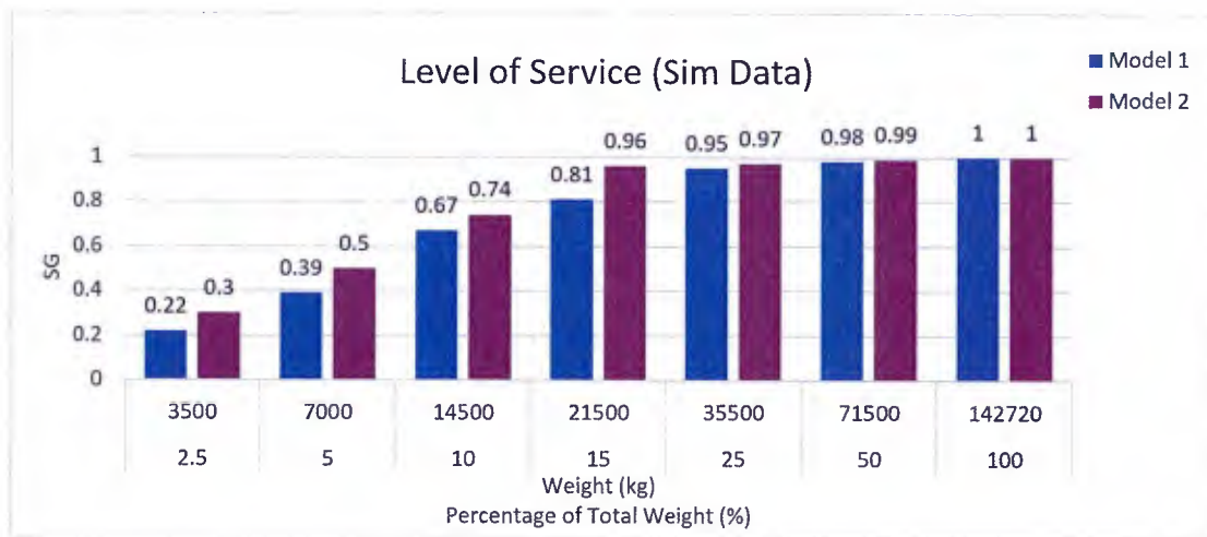
Figure 6.2: SG of Sim Data for different weight capacities for Model 1 and Model 2.
