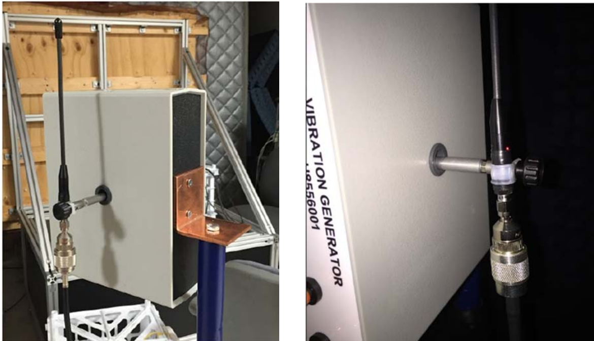
Figure 28: Monopole antenna attached to a vibration table.
