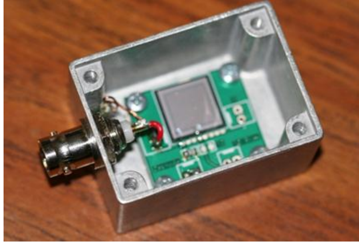
Fig. 3.9. Picture of the enhanced-performance silicon PIN-type radiation detector, when bound by aluminum/aluminum contacts. The active area is 1 cm 2 .
