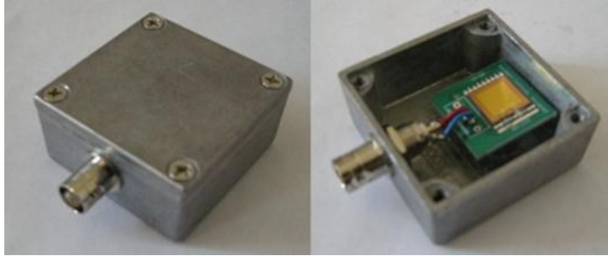
Fig. 3.2. Pictures of the fabricated silicon PIN-type radiation detector (right) and shielded module (left) for low energy gamma spectroscopy. The active area was 1\text{cm}^2 .
