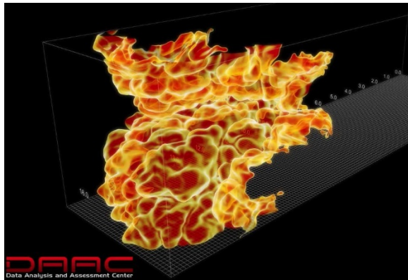
Structure of a hydrogen-air turbulent flame formed in the decaying upstream turbulence.
