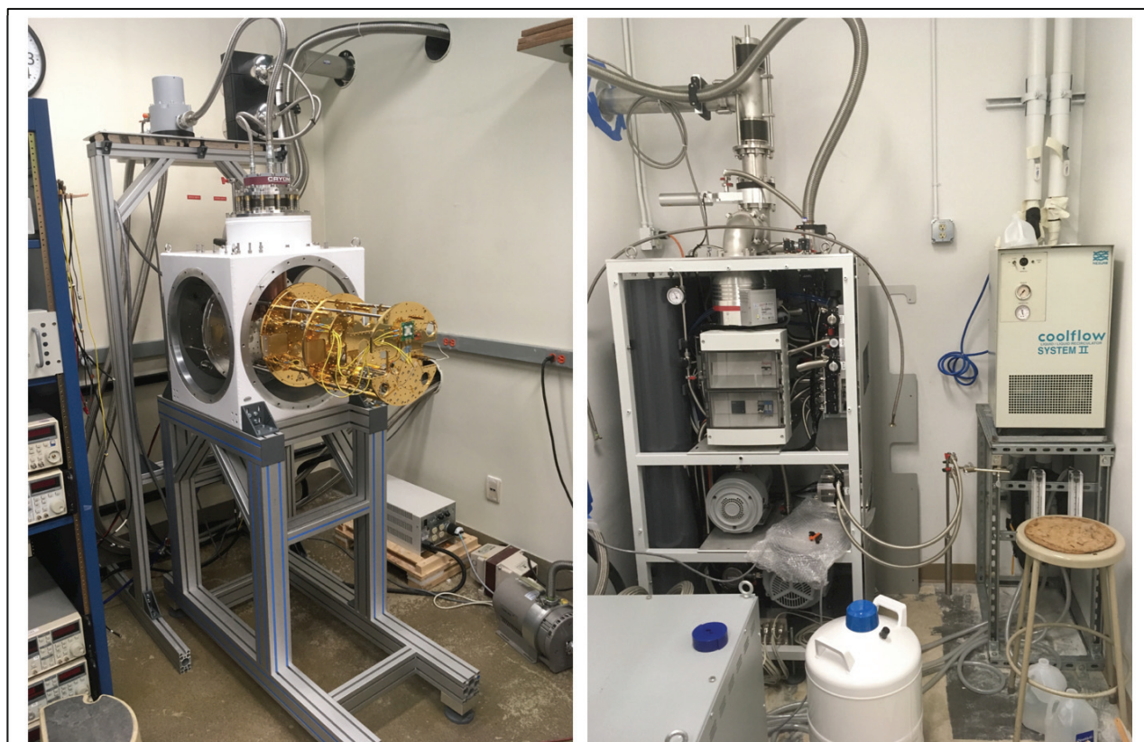
Figure 1. Cryogen-Free Dilution Refrigerator System. (Left) Cryostat and dilution unit with vacuum can and radiation shields removed. Note that this picture was taken before the full system wiring was installed. (Right) Automatic gas handling system, heat exchanger for cooling water, and cryocompressor (bottom left corner).
