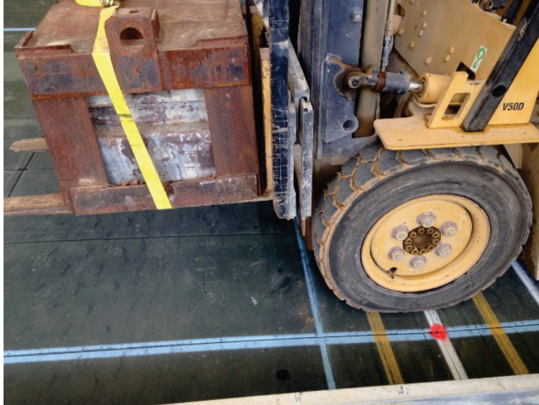
Figure 3.20. Loaded rut depth measurements.
