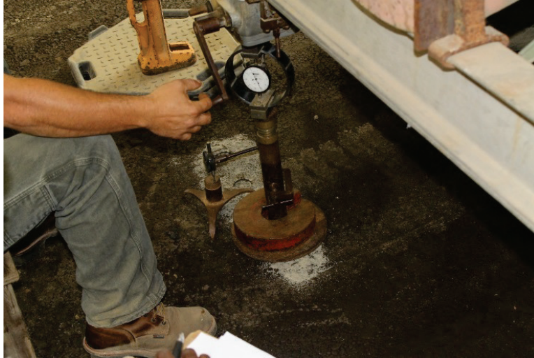
Figure 3.5. In situ CBR test.
