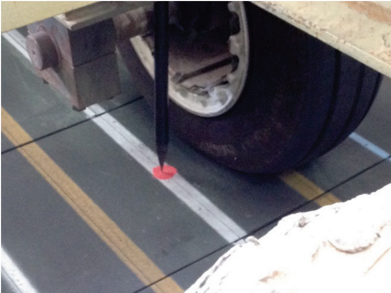
Figure 3.18. Elastic deflection measurement during trafficking.
