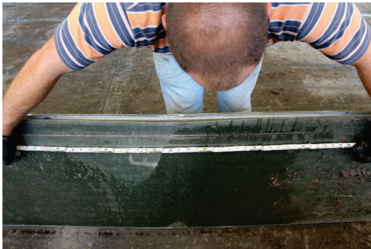
Figure 5.4. Two large bottom skin tears on panel 8.
