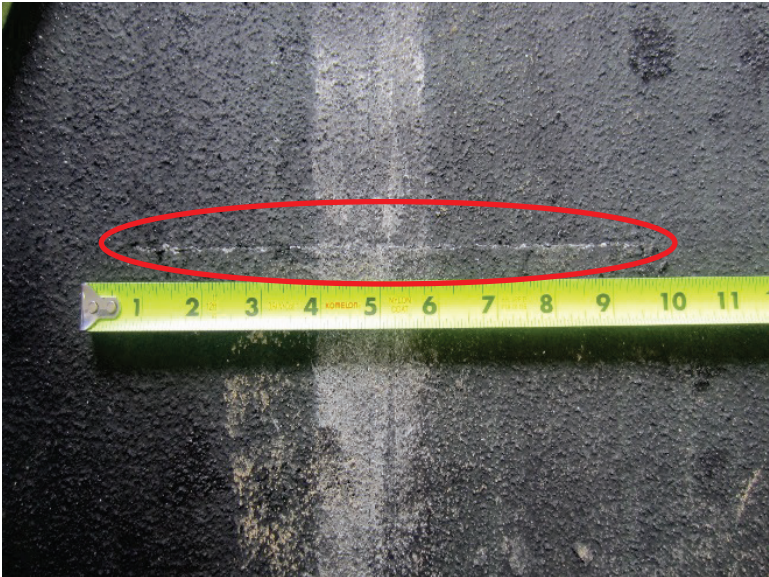
Figure 4.3. Top skin tear on panel 8 at 6,100 passes.
