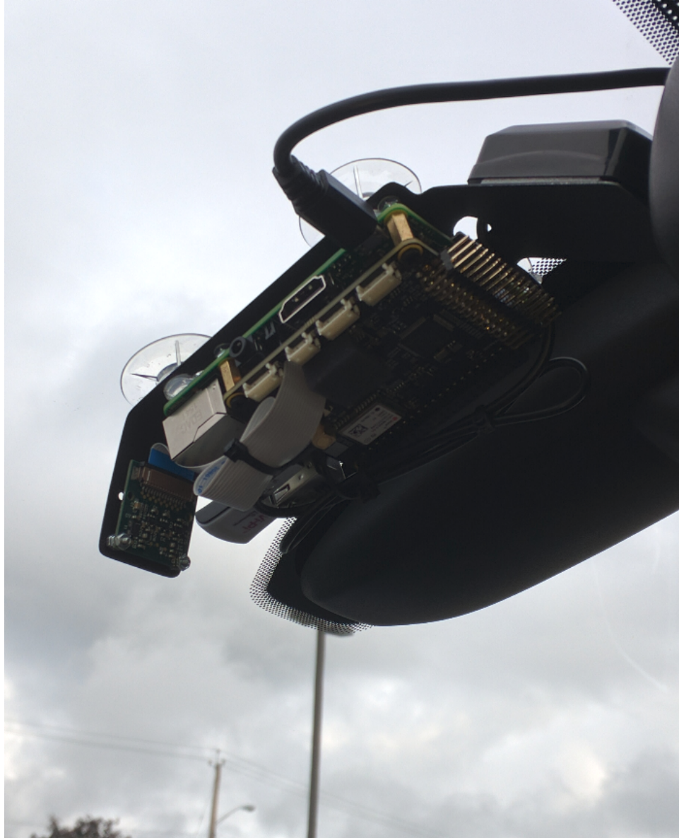
Figure 48. Test hardware mounted to vehicle windshield for collecting evaluation dataset as dashboard camera.
