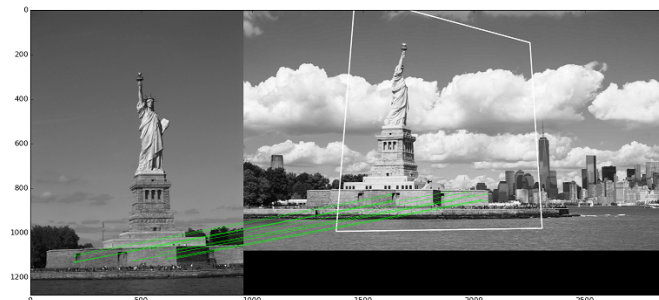
Figure 20. Matched visual features and associated perspective transform between images of the Statue of Liberty.
