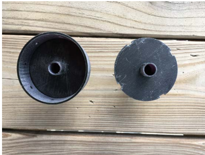
Figure 51. Side-by-side comparison of initial design (left) and revised design (right) of Base Plate
