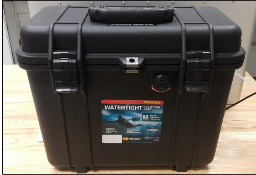
Figure 8. MarkOne 3D Printer Nylon Dry Box
