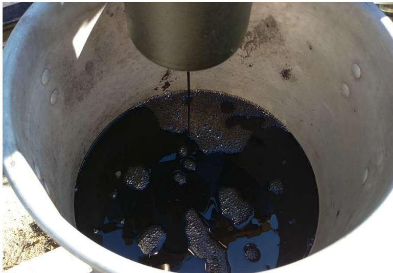
Figure 20 - Waste Drained from Clogged Fuel Filter
