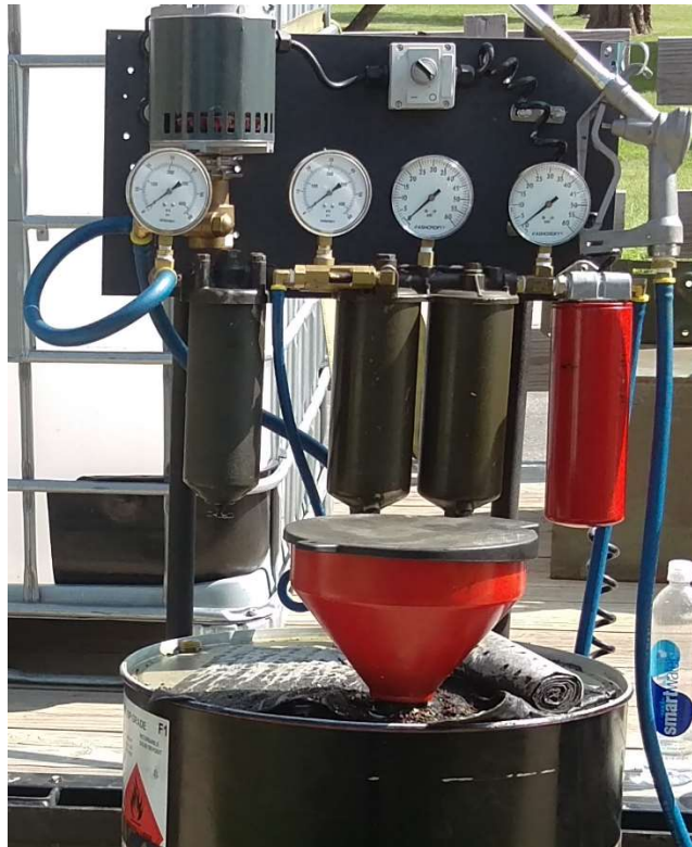
Figure 18 - WMO Collection Barrel with Cartridge Filter Rig
