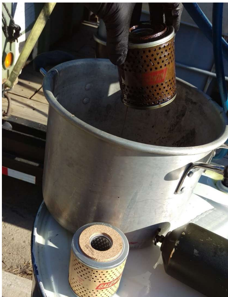
Figure 21 - Dirty Fuel/Water Separator Cartridge
