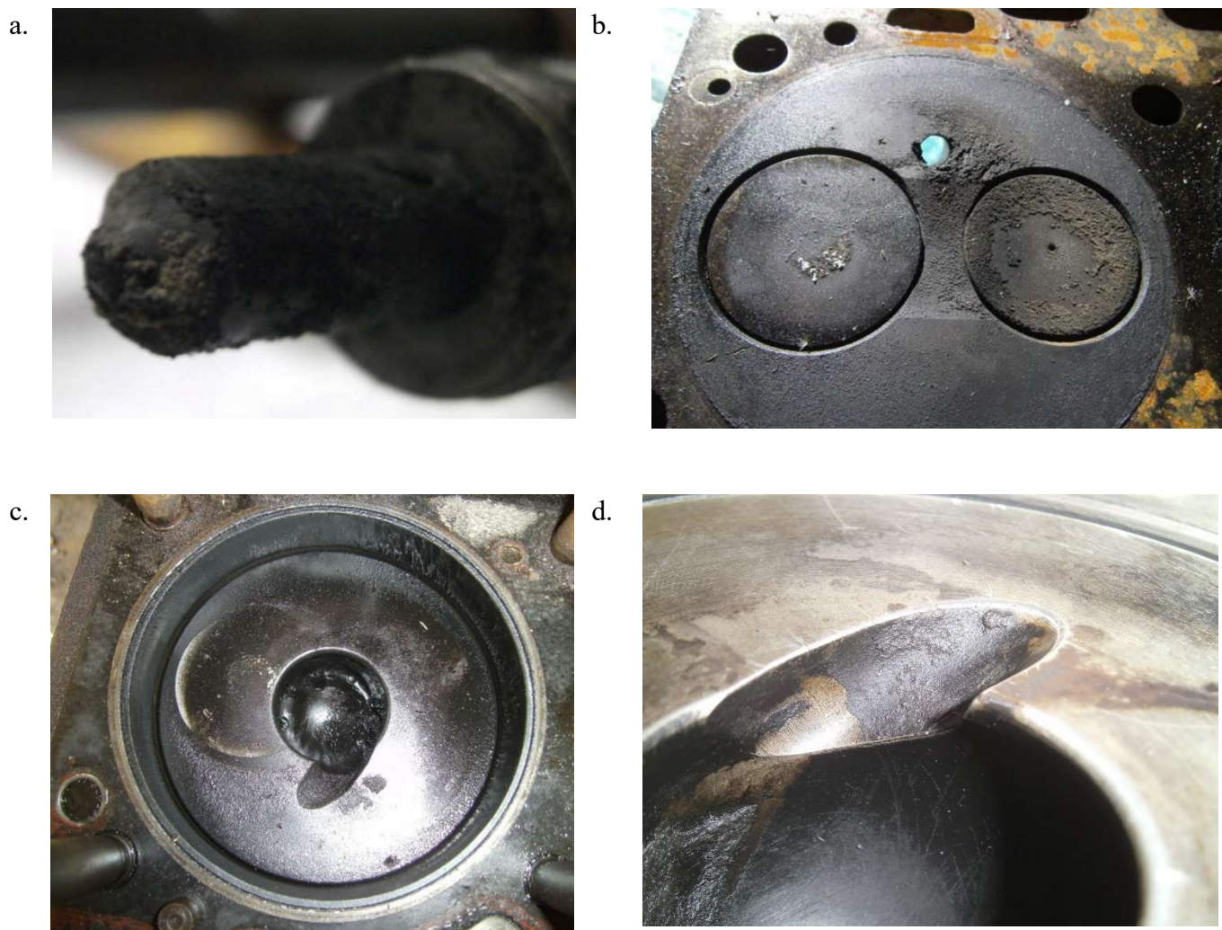
Figure 11 - Effects from WMO Blends on LDT-465 Components (Duncan, 2014)
