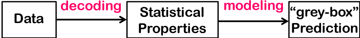
Figure 1: The “grey-box” statistical framework, where the statistical properties that we have investigated include Long Range Dependence, Extreme value, and Dependence. These properties are used to guide the design of statistical models for predicting cybersecurity situational awareness from various aspects (e.g., cyber attack rates). “Grey-box” means that the prediction models are devised to accommodate the statistical properties exhibited by real-world data.
