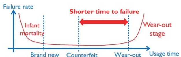
Fig. 2. The classical bathtub curve illustrating typical device failure characteristics.
