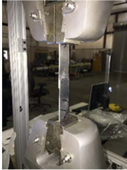
Figure 10: Lap shear specimen in the Instron.
