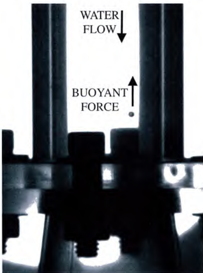
Figure 3.1.20 Image of a 1.3 mm gas bubble stabilized in the DOS water tunnel.
