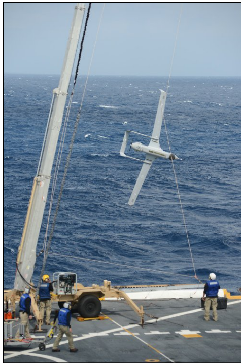
Figure 1. RQ-21A Captured On Shipboard Using SRS. Source: Federation of American Scientists (2000, 1).
