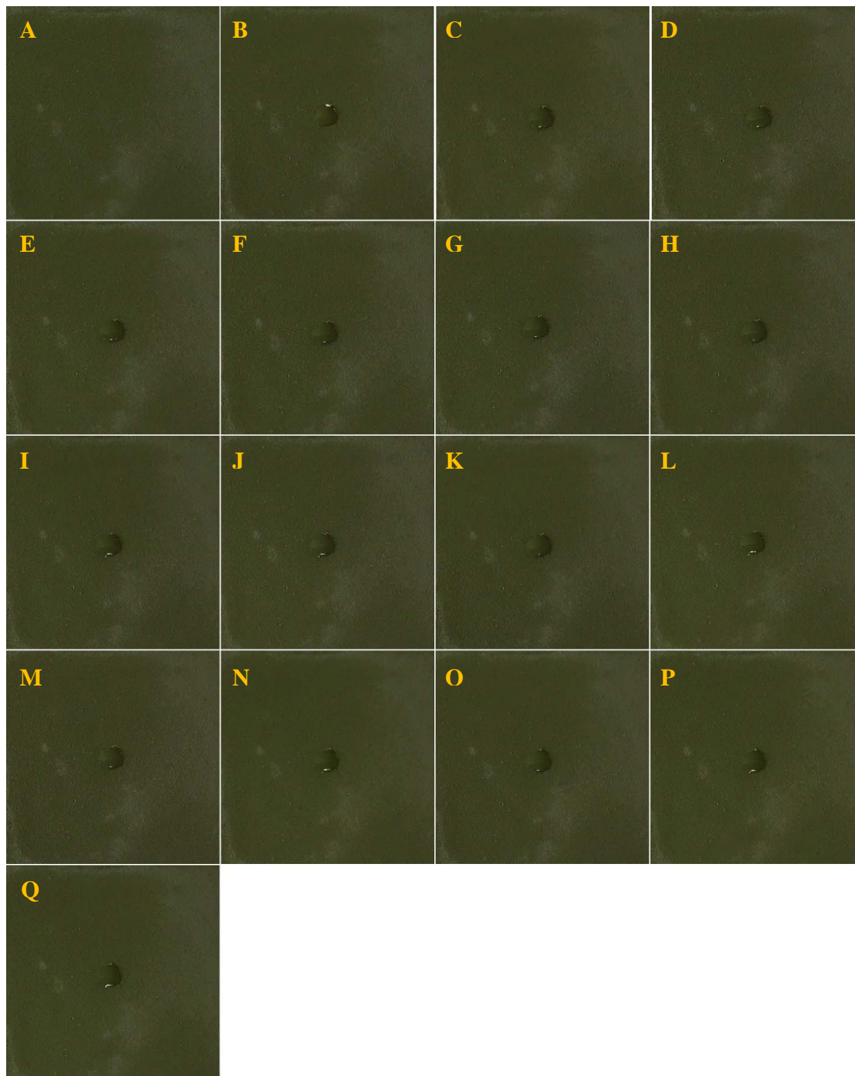
Fig. A15 — DMMP on the porous polymer with no lubricant. Images of a coupon before application (A) and at 0 (B), 0.5 (C), 1 (D), 1.5 (E), 2 (F), 2.5 (G), 3 (H), 3.5 (I), 4 (J), 4.5 (K), 5 (L), 10 (M), 15 (N), 20 (O), 25 (P), and 30 (Q) min following application of the target
