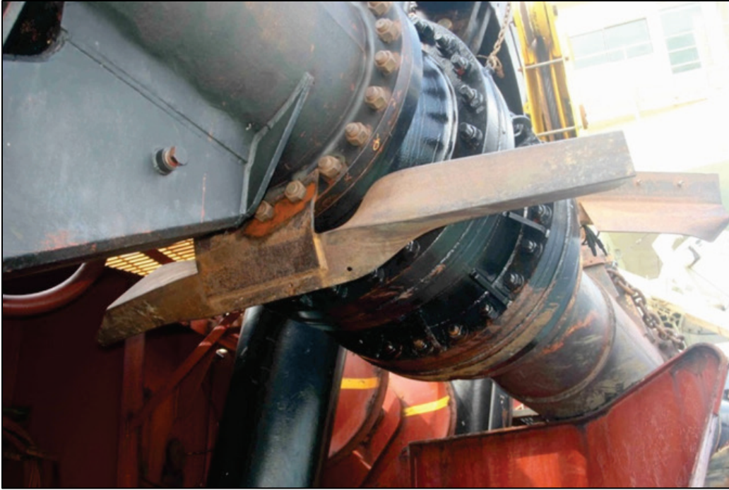
Figure 6. Damage to portside chain bracket and acoustic camera mount.
