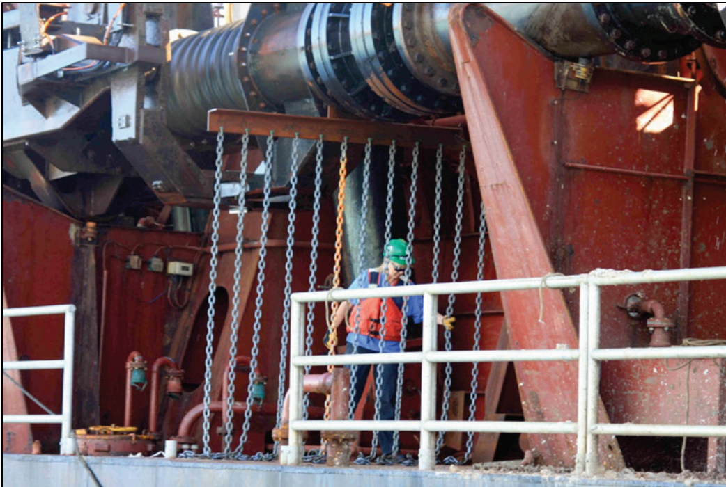
Figure 21. Endangered species observer inspecting condition of TTC after dredging a load on the Essayons .
