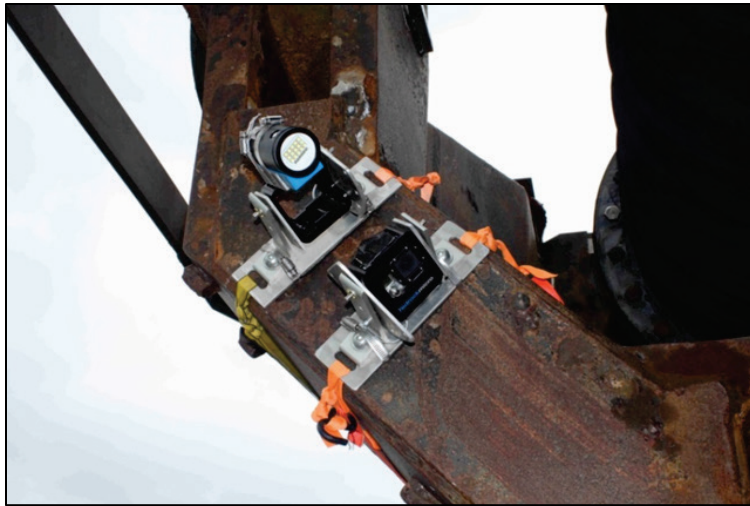
Figure 2. GoPro camera in underwater housing and 700-lumen light source mounted on outboard gimbal frame of the dragarm.
