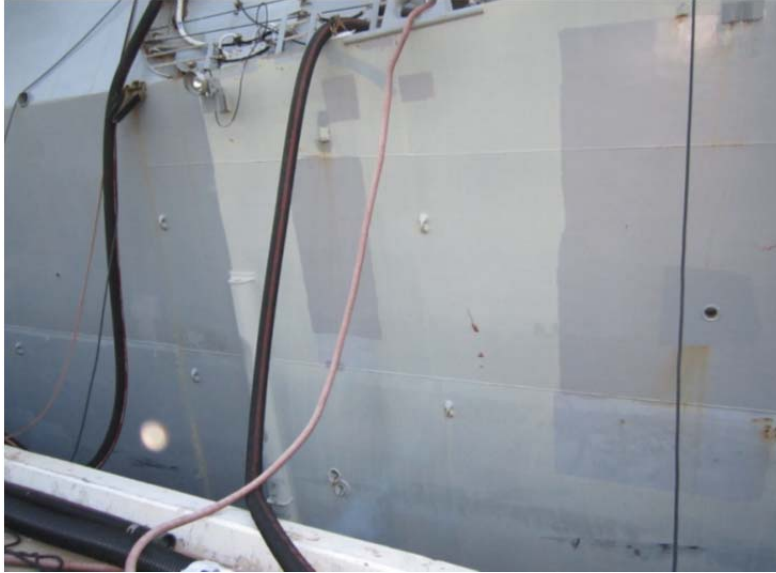
Figure 3. Quilt Pattern of Paint on a Ship. Source: Naval Supply Systems Command (2017).
