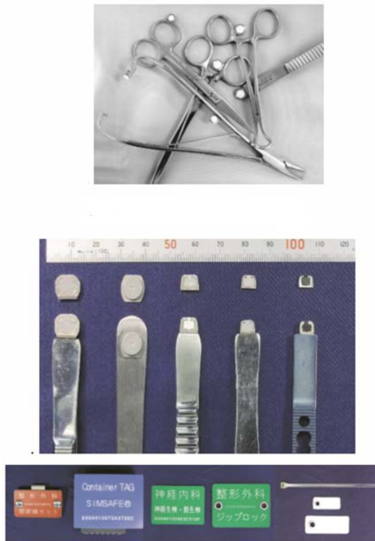
Top: Various kinds of housed RFID tags that are welded to the instruments. Bottom: RFID tags that are attached to the containers, baskets, and small instruments.
