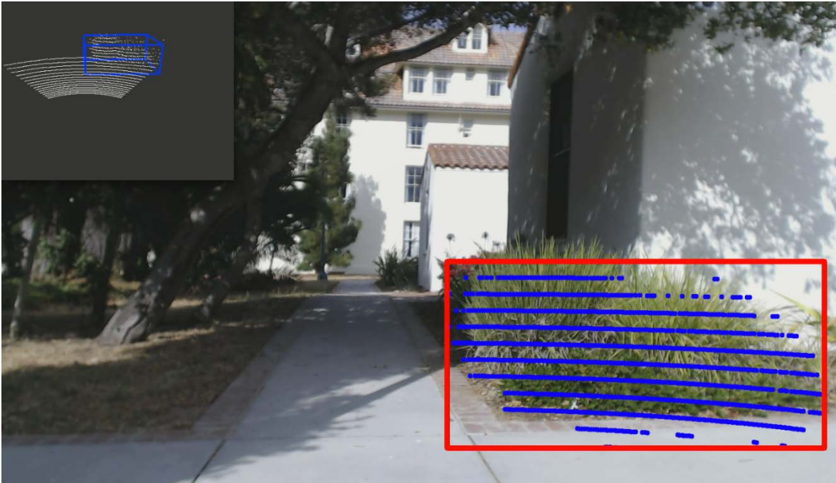
Figure 22. Implementation of 3D-2D Correlation of 3D Pointcloud Segment to Bounding Box on 2D Frame
