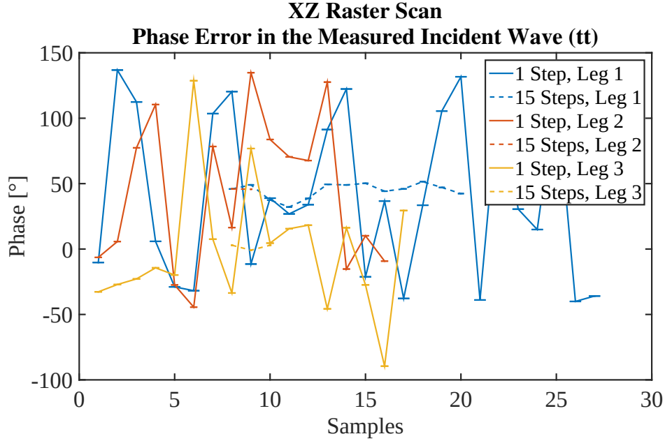
Figure 36. Phase errors (tt) in the incident field measurement of all legs of the x and z raster scan measurement with the Vicon TM uncertain error bars applied
