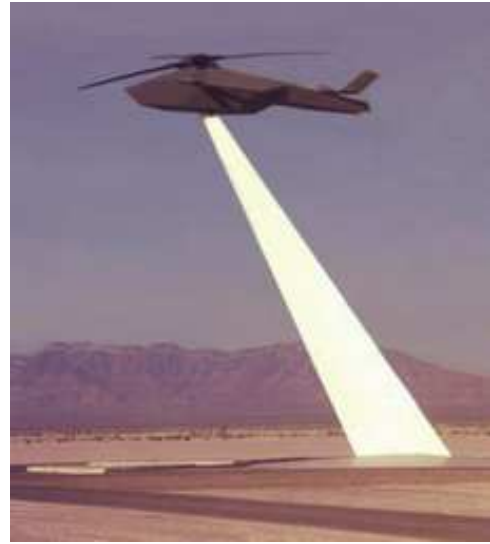
Figure 1. Low-Observable helicopter prototype model being measured at NRTF [4]
