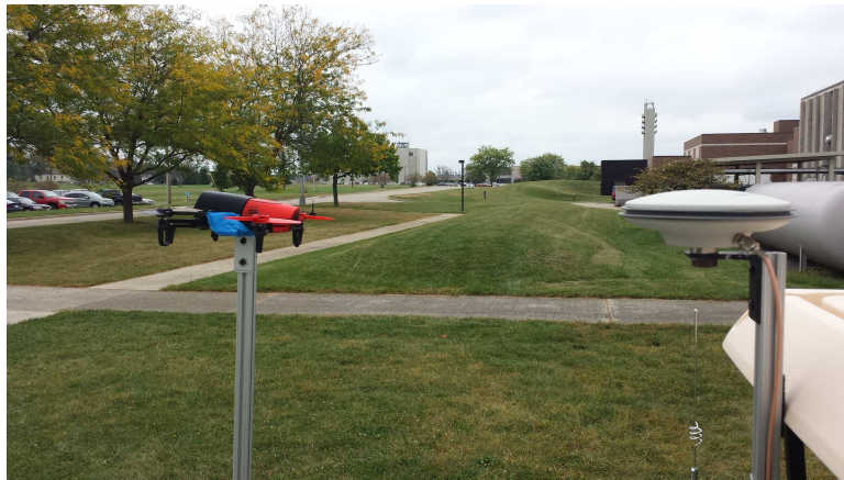
Figure 14. Bebop Quad-rotor Mounted on Golf Cart for GPS Characterization
