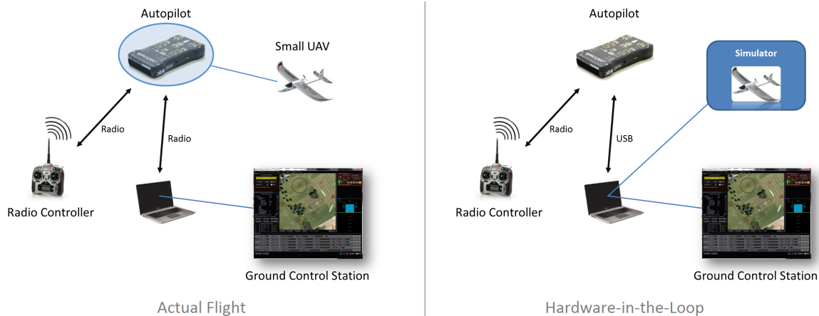
Figure 4. Hardware-in-the-Loop. The setup on the left shows how small UAVs are typically controlled in the hobbyist community—an operator provides manual RC inputs while passing commands and updating parameters via GCS (both over radio). On the right, the operator controls the simulated vehicle in the same manner. However, the embedded system (i.e. hardware autopilot) communicates with the simulator over a serial/USB connection, with the GCS acting as an interface between the two.
