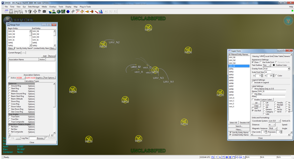
Figure 23. SIMDIS Overview. SIMDIS intercepts and interprets the DIS packets broadcasted by the simulation. The Range Tool on the left provides ranging information (i.e. difference in altitude, slant range, etc.) between two or more entities while the Super Form on the right provides view customization (i.e. adding/removing labels, data tables, local grids, etc.) and the ability to focus the view on a specific entity. The main window provides point-and-click interactivity, allowing users to pan, tilt, and zoom freely while the simulation is running.
