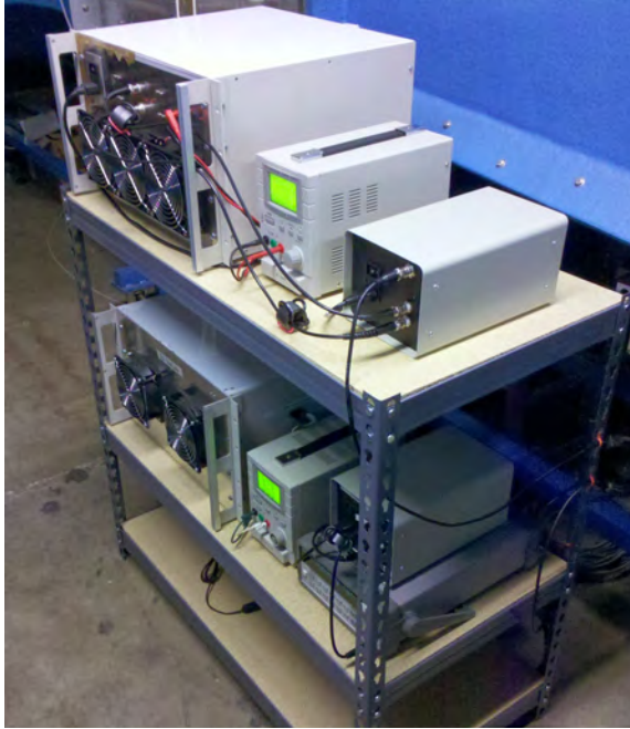
Figure 3.5: Nanosecond pulse generators located inside of the tunnel loop. From left to right: main unit, low-voltage DC power supply, control unit. High-voltage DC power supply not shown.
