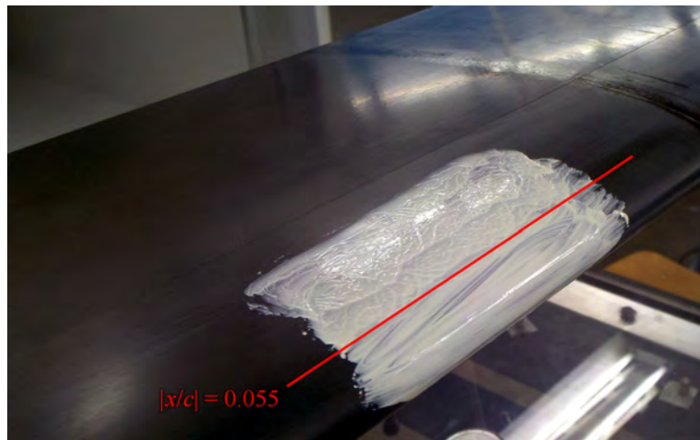
Figure 4.2: Surface oil flow visualization indicating the separation line.
