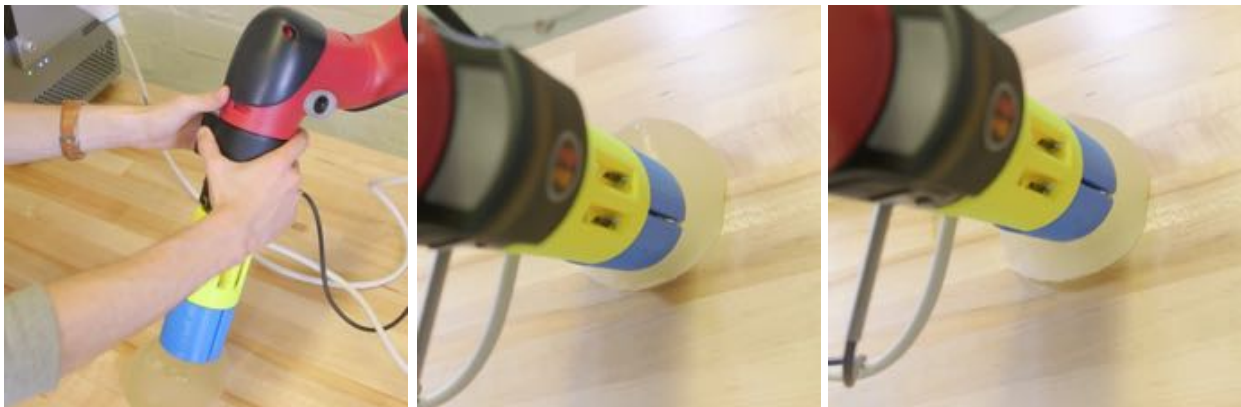
Figure 5: Time sequenced images of lateral end-effector motion under a constant force setpoint on a physiologically inspired phantom.
