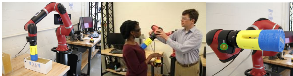
Figure 1: Images illustrating the research platform we are developing for investigating technologies on robotically-assisted medical ultrasound. The platform, which consists of a robotic manipulator, force/torque sensor, ultrasound transducer mount, and haptic interface device, is shown in the leftmost image. In one approach to human-robot interaction that we are investigating a person (called the “spotter”) positions and orients the ultrasound transducer to a point of contact on a subject as illustrated in the center image. The hybrid force/velocity control is then engaged with a button on the wrist cuff of the robot as illustrated in the rightmost image (highlighted in green oval).
