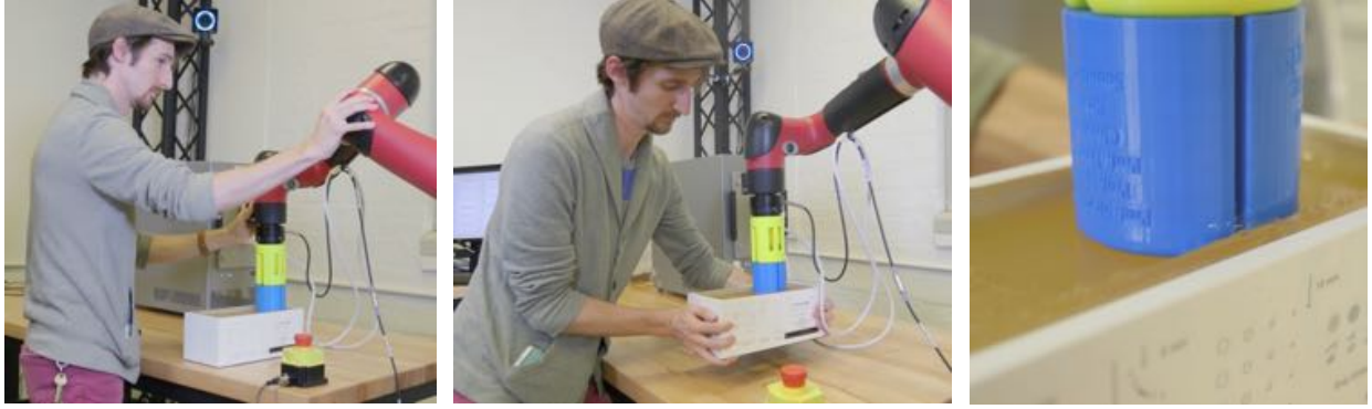
Figure 3: Illustrations of experiments to evaluate the performance of the force/velocity controller subject to displacements of the phantom, simulating movement or respiration of the subject.
