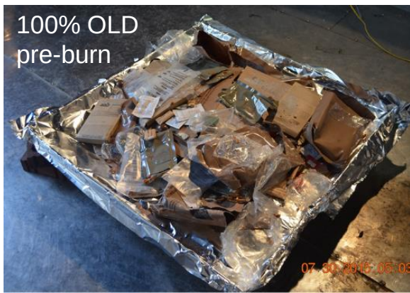
Figure 13. Fiberboard and MRE Test Material on 3.2 × 3.2 foot Steel Plate
