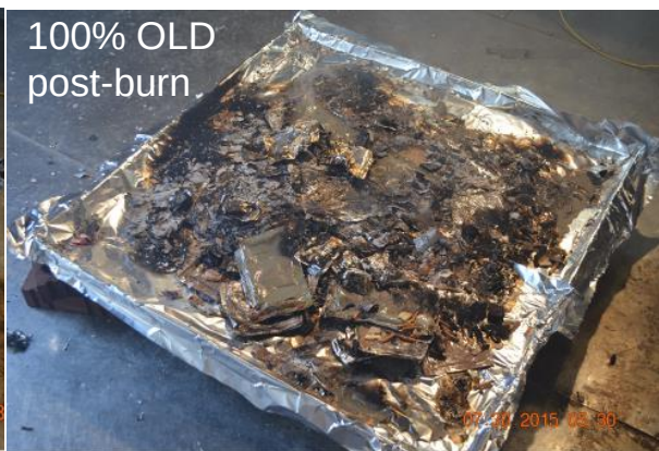
Figure 13. Fiberboard and MRE Test Material on 3.2 × 3.2 foot Steel Plate
