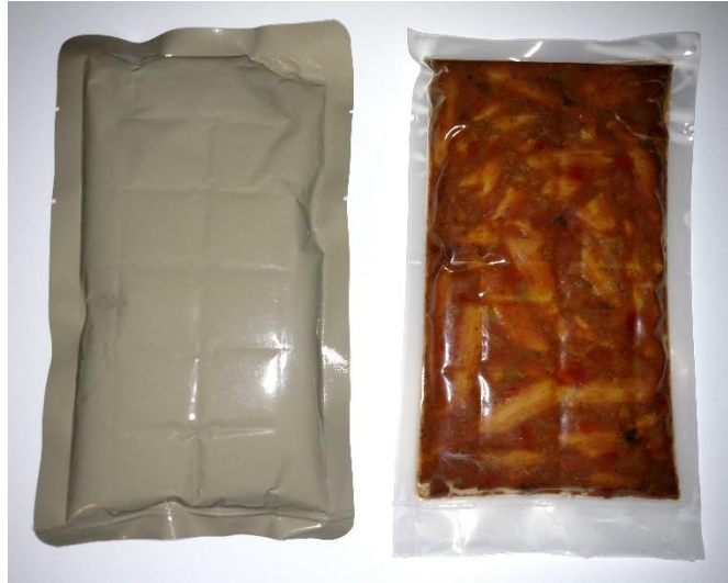
Figure 27. MRE Aluminum-based versus Nanocomposite-based Primary Packaging
